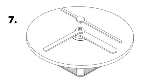
Please be careful not to destroy your clock movement by removing the second hand after it is fitted! The second hand fits VERY tightly and is NOT intended to be removed after fitting as this can pull the metal hand spindle out of the movement which WILL destroy the movement. For this reason please don't push it on to the spindle too tightly, especially if you may want to remove it again.
