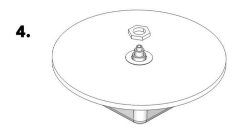
Please be careful not to over tighten the nut as this can distort the cogs in the movement and stop it from working.
