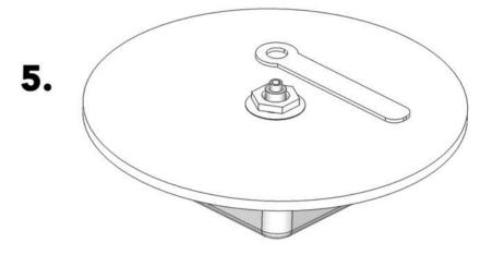
Turn and wriggle the hour and minute hands whilst gradually pushing them onto the movement spindle, making sure they are pointing to the 12.
